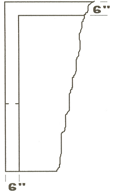
PARTIAL SECTION THROUGH SIDE WALL
